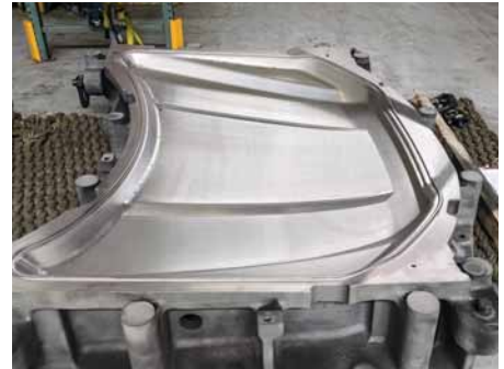
Fig. 4. Stamping die after plasma nitriding
