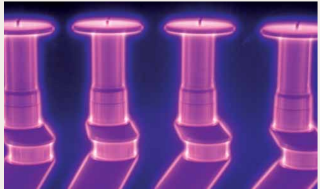
Fig. 5. Ion nitriding of the crankshafts for aerospace applications; note masking plates on top of the crankshafts.
